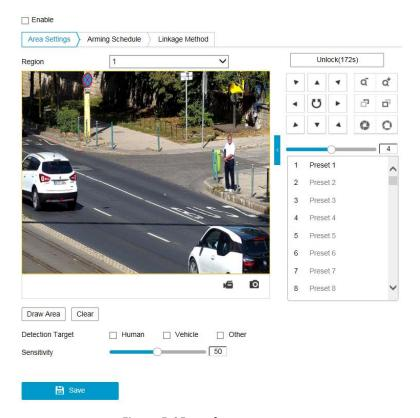
Figure 5-25 Configuring Region Exiting Detection
