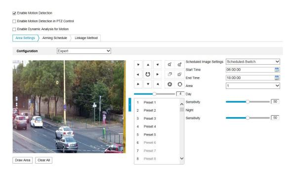
Figure 5-10 Motion Detection Settings-Expert
