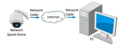
Figure 2-5 Accessing the Camera with Static IP Directly
