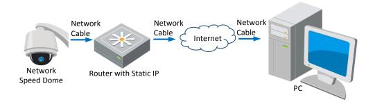
Figure 2-4 Accessing the Camera through Router with Static IP
