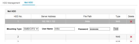
Figure 5-5 Select Net HDD Type
