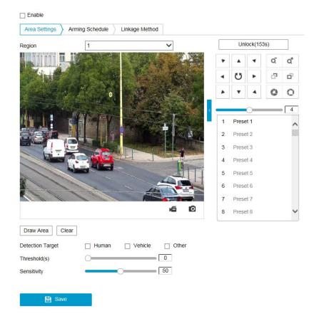
Figure 5-22 Configuring Intrusion Area
