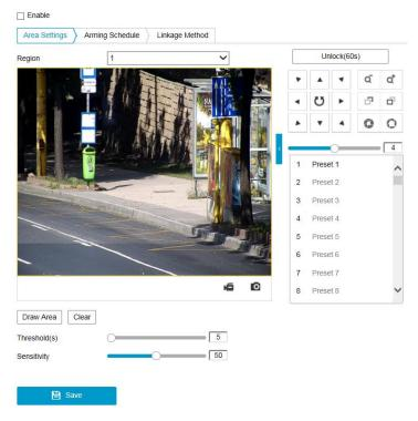
Figure 5-26 Configuring Region Exiting Detection
