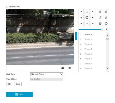
Figure 5-29 Configure the PTZ Limit
