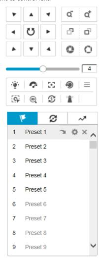
Figure 4-4 PTZ Control Panel
